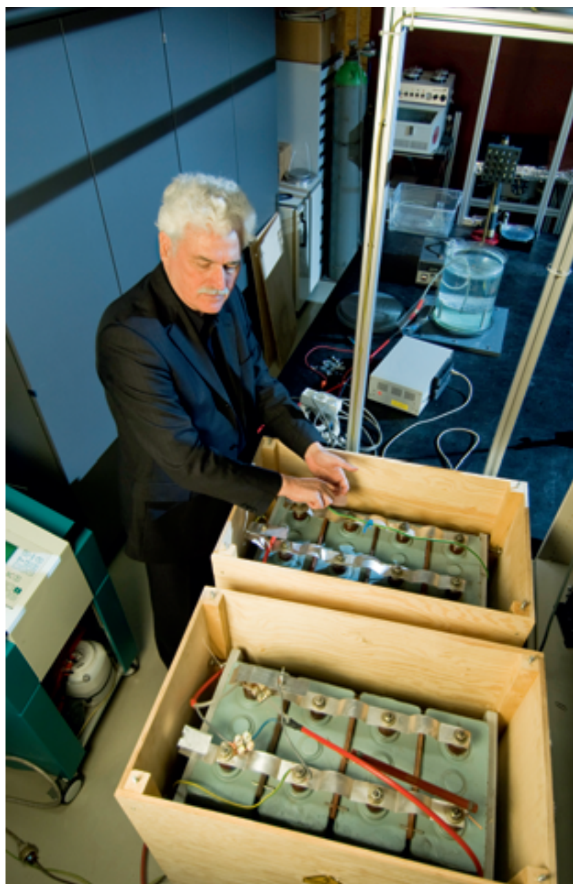
Tension-filled: This condenser bench generates 5,000 volts. Gerd Fußmann attaches the electrodes that will vaporize and ionize a water droplet.
